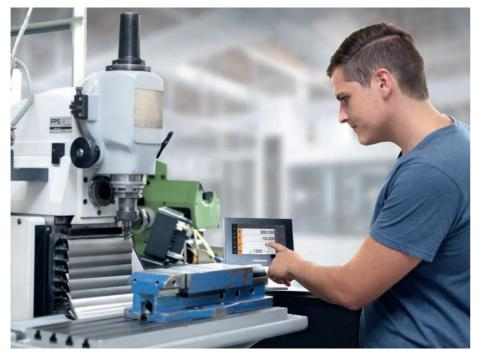
Presets can be found fast and accurately with an edge finder. The ND digital readouts support you with special probing functions.
